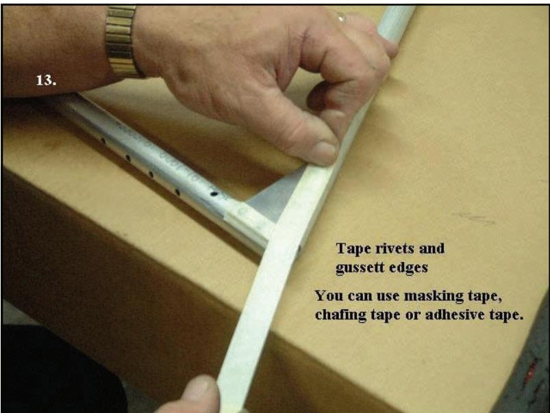
Don't apply too much tape, especially on the outer perimeter of the frame. You'll need good, clean surfaces for the glue and fabric to stick to.
