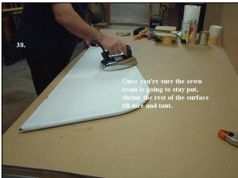
We are getting close to completing the heat shrink process for this panel. Carefully iron out any last remaining wrinkles and folds - Avoid applying heat to the overlapped edge.
