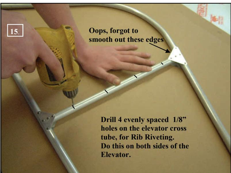
Don't forget about the cross tube on the elevator. Sand and clean, ready for glue. It looks like Dave forgot to smooth out the edges of that gusset. All sharp edges must be smoothed out.
