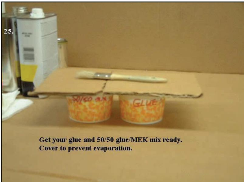
A scrap piece of cardboard works well to cover the bowls and prevent evaporation.
