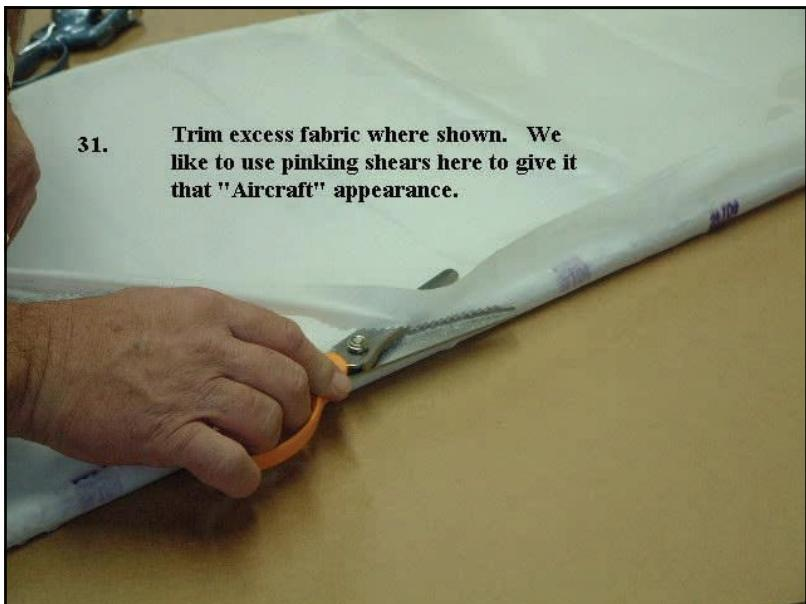
Take care when cutting the fabric. The neater the cut, the better the final appearance will be when it's on the plane. You can opt to have the cut edge on the underside of the stab and elevator for better appearance.
