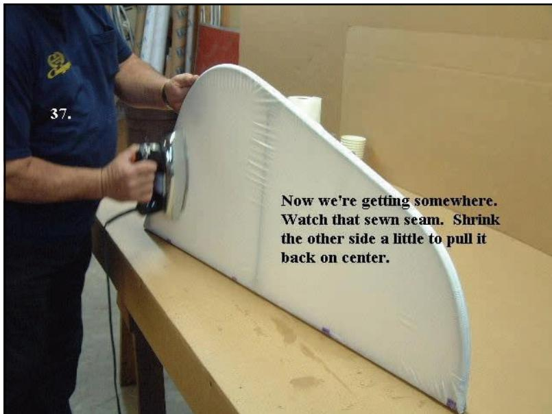
Apply 'even' amounts of heat on both sides of the frame.
