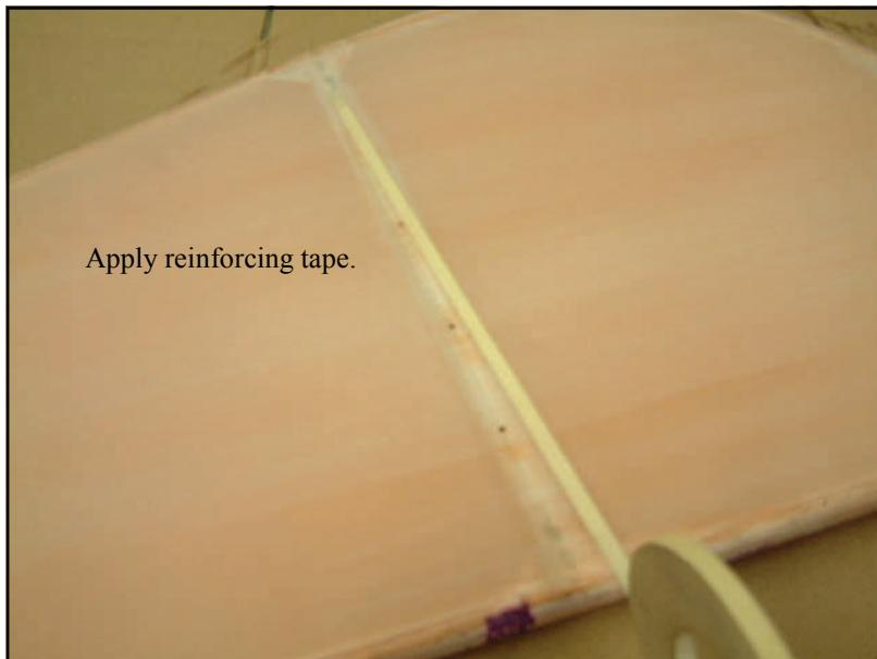
Carefully align the tape along the centerline of the holes. Cut to length and stick the tape down on the tube.
