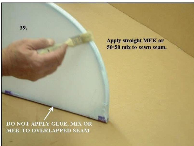
At this point, the sewn seam should be fairly straight and even. Apply some 50/50 mix to the seam.
