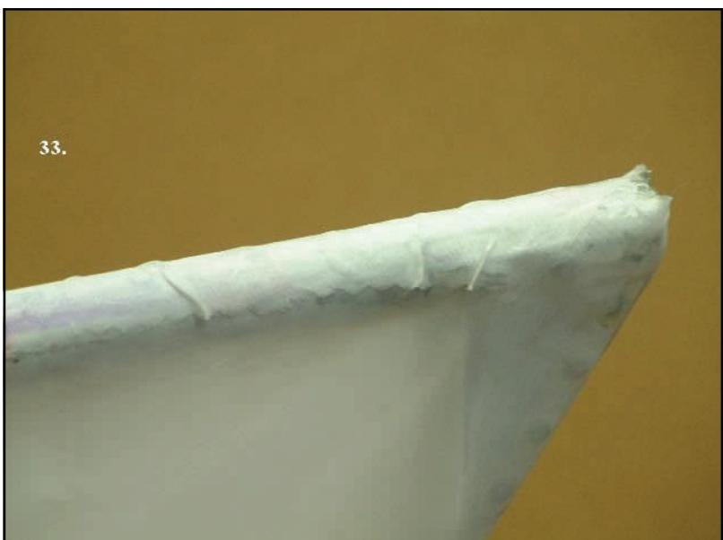
Even the professionals end up with a wrinkle or two. These can easily be removed with the iron before heat shrinking..
