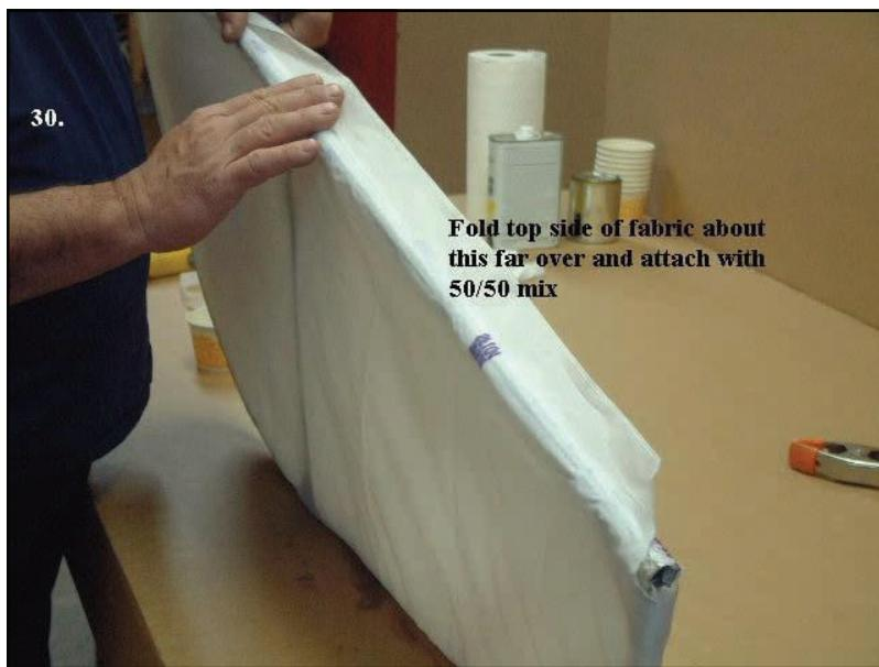
As before, make sure the 50/50 mix soaks through the fabric and re-activates the 100% glue previously applied.
