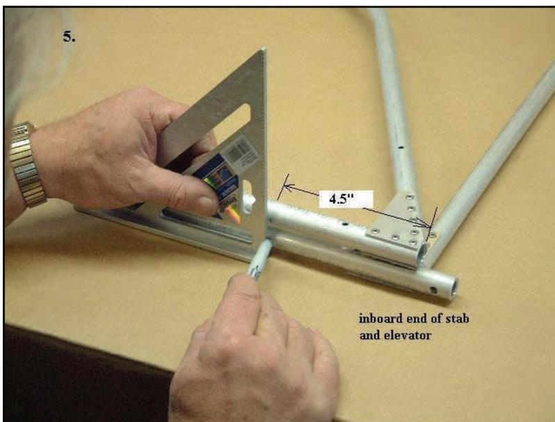
NOTE: the elevator is shorter than the stab.
