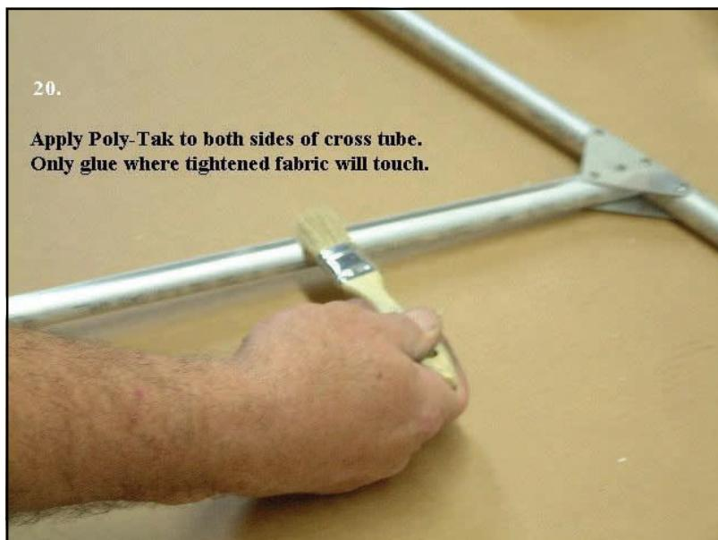
Running the brush 'flat' along the cross tube (as shown) will put just the right amount of glue needed for the covering process.
