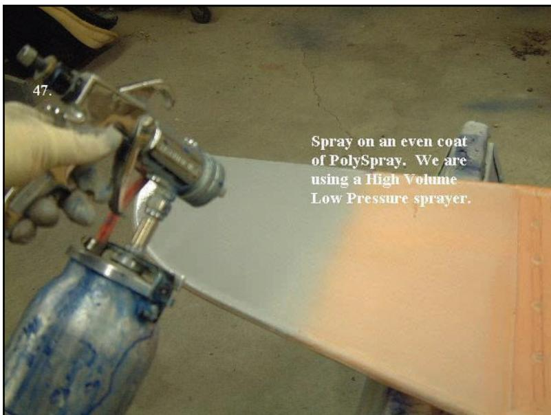
The key here is smooth and even strokes with the spray gun. Spray off the edge of the panel before shutting the spray gun off. Do not apply thick coats. Thinner coats dry quicker and are easy to fill, if required, with another 'THIN' coat.
