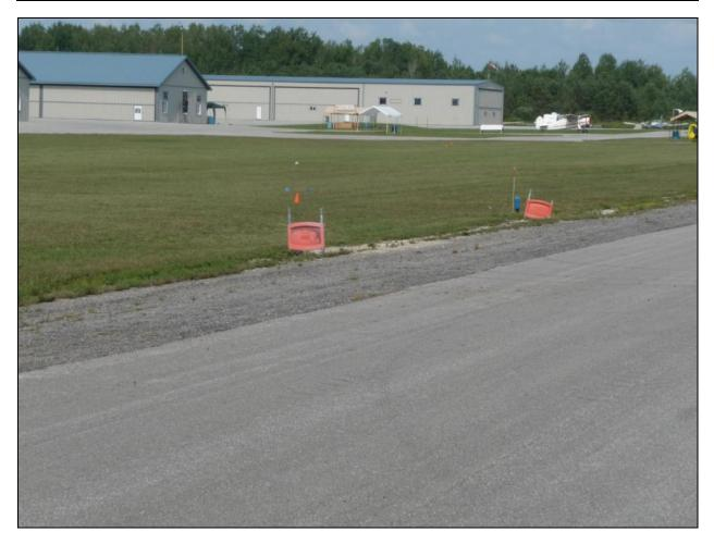
After exiting the runway you will be directed to your parking spot. Please follow the directions of our staff. Aircraft will be parked with nose facing RWY 26. There are lines cut in the grass which we will be placing your main gear on. This will keep sufficient clearance between aircraft which creates lanes which you can use for departure. (see the photo below).
