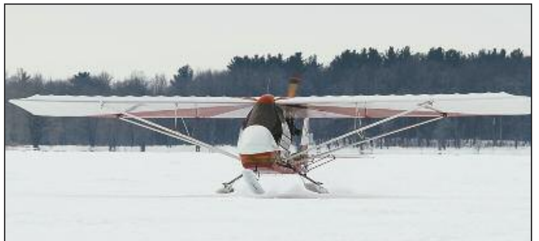
This classic Challenger long wing looks hesitant to touch down. No worries mate – the ice is 14 inches thick – enough to support an eight to 10-ton truck!
