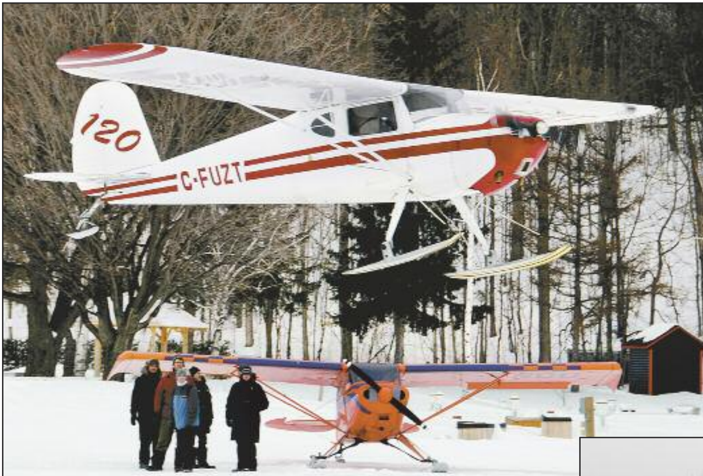
At left: C-FUZZ is a two-seat 1946 Cessna 120. The Cessna 140 is a 120 with flaps. The Cessna 170 is a 140 with four seats and a bigger engine. These are the direct ancestors of the ubiquitous 150 and 172. Today, a new Cessna 172 costs US$364,000! Photos courtesy Jean-Pierre Bonin
