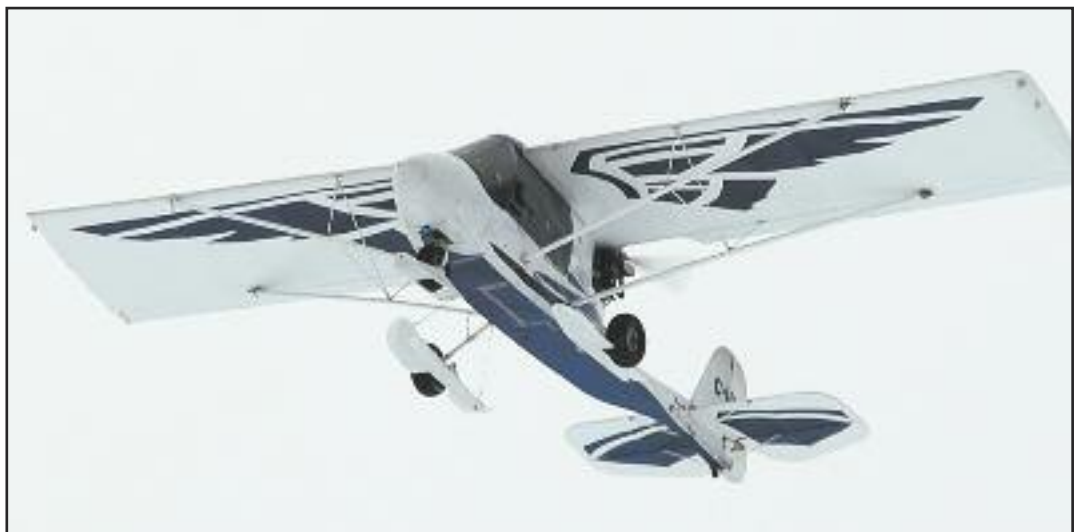
Above left: This 1961 Piper PA-22-108 Colt was converted from tricycle to conventional gear. The taildragger configuration makes a plane with the engine in the nose much more practical on skis.
