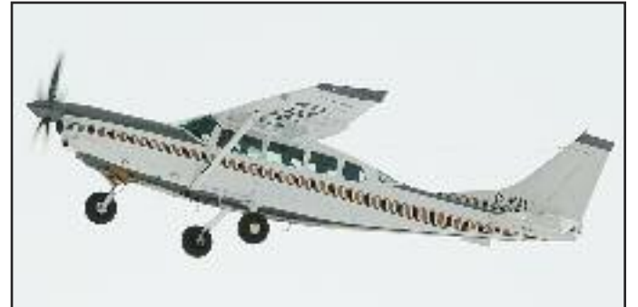
This Cessna 207 has been modified with a turbine engine and a five-bladed prop. With all that power it still couldn't land because conditions were only suitable for skis.
