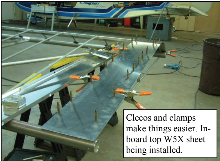
Pre-drilling W5X sheets makes life easier. Four inch rivet spacing works well.
