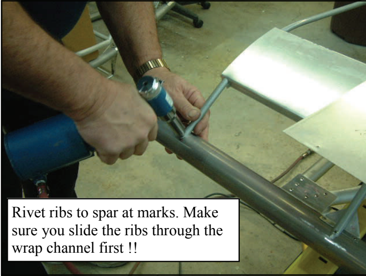
Slide ribs through channels before riveting to spars.
