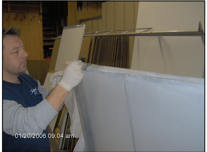
Flat sheets (W5X) top and bottom make good anchor points for the fabric.
