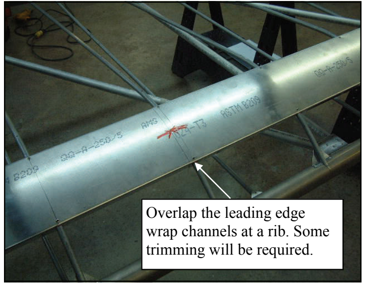
Rivet rib tip with long stainless first
