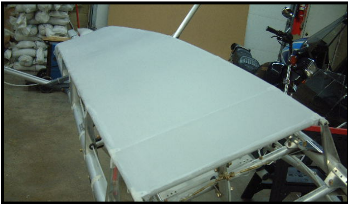
Bottom fabric glued to the bottom stringer assy. Do not 'over shrink' as bowing of stringer may occur
