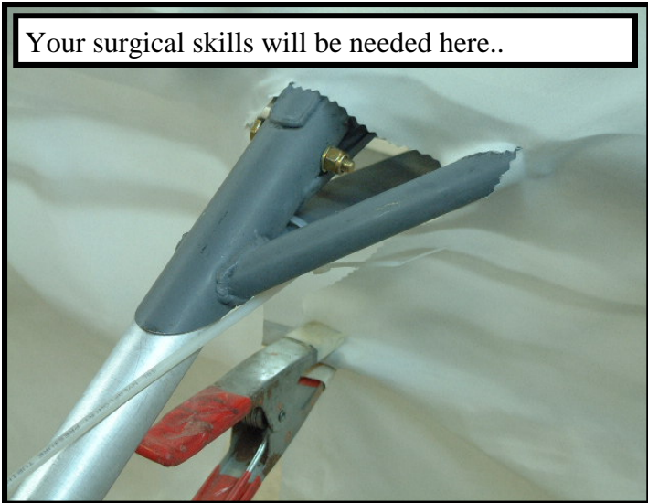
Bottom fabric glued to the bottom stringer assy. Do not 'over shrink' as bowing of stringer may occur
