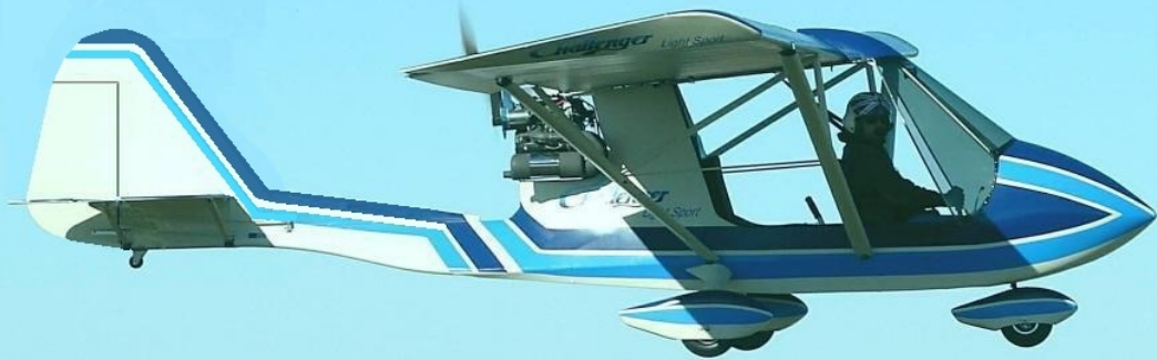
LSS-XS-50 with Rotax 503 (52 hp) represented in this photo.
