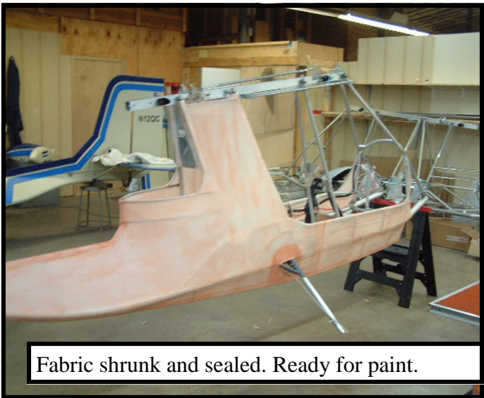
A pre-shrunk and shaped collar here will tidy up the gear leg weldment area. Use Poly-brush to apply.
