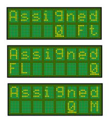
When the **Altitude** option of the mode menu is set to Feet, the **Assigned** altitude is adjusted in feet.
