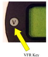
To bring the stored VFR code to the standby line press the **ENTER** key then the **VFR** key.
