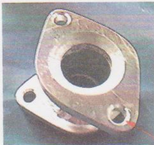
Portside transition flange
