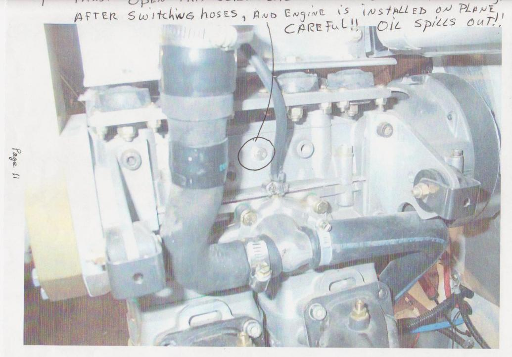
You must open this bolt to bleed the Rotary valve oil into the case. Critical to do! Carefully open until oil starts to trickle out. Do not over tighten when reinstalling.
