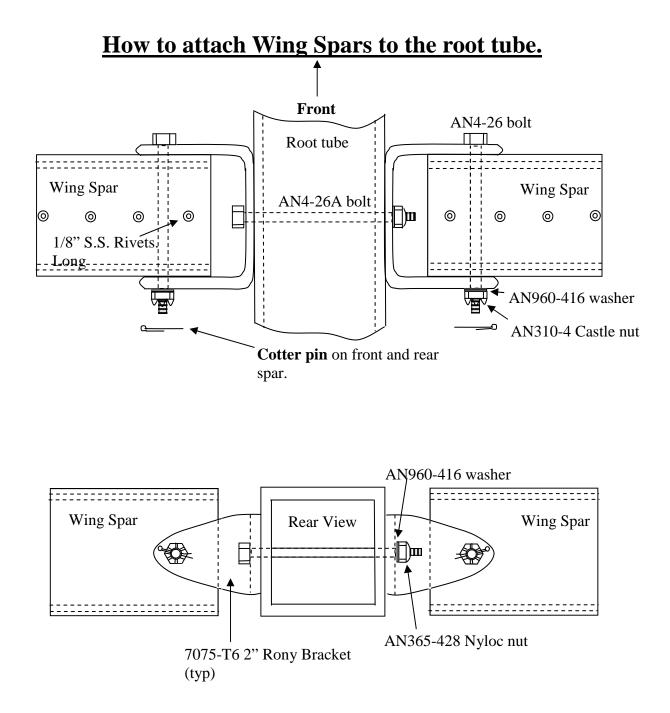
Install wing spar and strut attach brackets as per illustrations.
