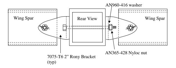
Install wing spar and strut attach brackets as per illustrations.
