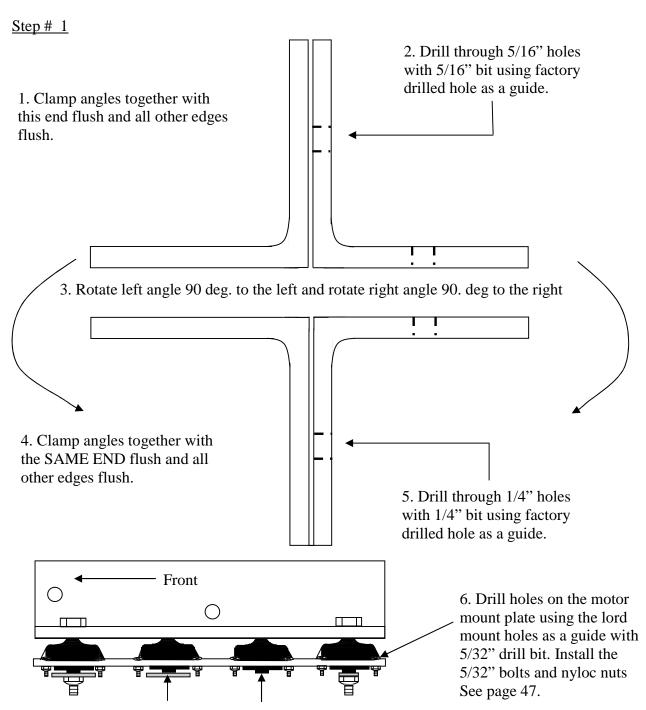
7. Drill remaining 1/4" holes through lord mount bushings with 1/4" drill bit. Be sure to install large area washers on the front 4 lord mounts
