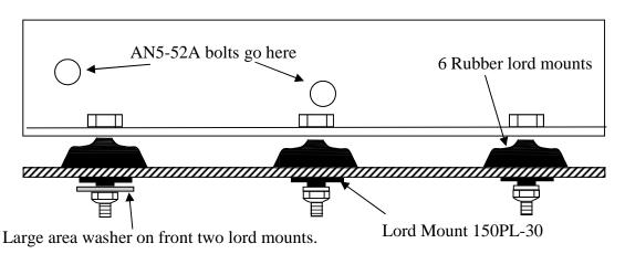
Attach the rubber Lord mounts to the engine mounting plate as shown on page 46. The Lord mounts are installed on TOP of the plate with the higher pointed end facing UP. The 5/32" holes will have to be drilled in the plate. Install the 8 (6 for Rotax 447) with the 32 x AN525-832R10 bolts and nuts provided.
