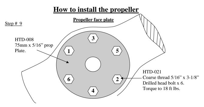
Install Propeller and prop plate with the 6 coarse thread 5/16 bolts (drilled head) provided. Be sure that the flat side of the prop is to the rear and the airfoil side of the prop is to the front. Tighten propeller bolts to (18 ft lbs.). **Tighten in sequence indicated above**. Try to tighten prop bolts equally to prevent propeller from being pulled out of 'track'. Safety wire prop (reference below) with wire provided. Since prop bolts are 'safetied', you need not use Loc-tite on threads.
