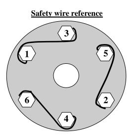
Bolt loosens by unscrewing to the left
