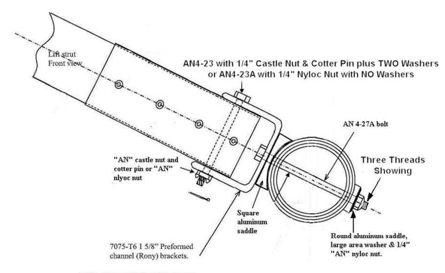
ALL BOLTS MUST BE INSTALLED EXACTLY AS SHOWN DO NOT OVERTIGHTEN NUTS
