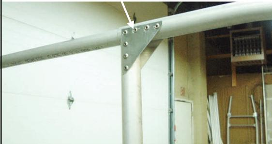
Remove the two shipping alum rivets, de-bur holes and insert extension tube. Adjust the extension tube accordingly to fit in line with the trailing edge of the rudder. Some trimming will be required at the end of the tubing to obtain a good fit.
