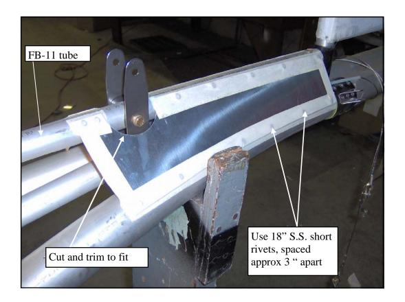
The FG-99 is designed to prevent the FB-11 tube from excessive movement. Once installed, but sure to work all edges and corners to a smooth finish. Cover the rivets and edges with tape, prior to applying glue and covering.
