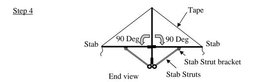
Use filament tape to hold the stabilizer surfaces squarely in place.
