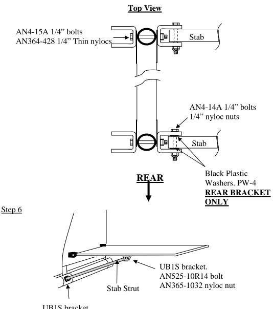
UB1S bracket. AN525-10R14 bolt AN365-1032 nyloc nut
