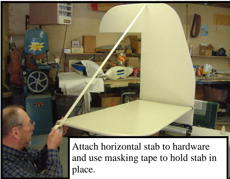
Attach horizontal stab struts to fuse.
