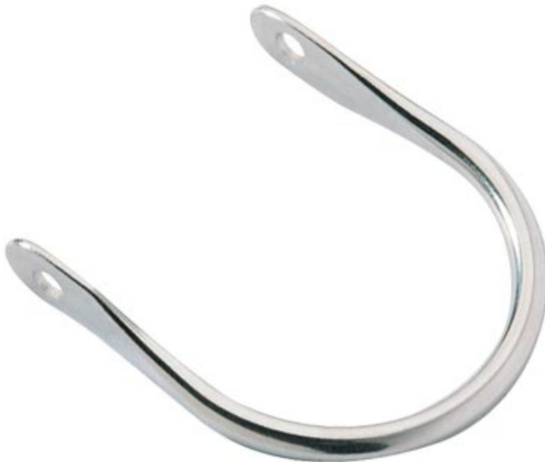
There are numerous sizes of boom bails! Get them 80mm (3 1/8") long and 65mm (2 1/2") wide with material diameter 6.4mm (1/4") having 2 x 6.6mm (1/4") diameter fixing holes.
